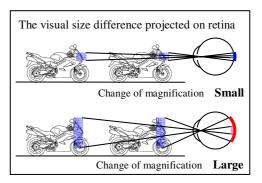
Figure 3. Principle of enhancing a sense of speed
